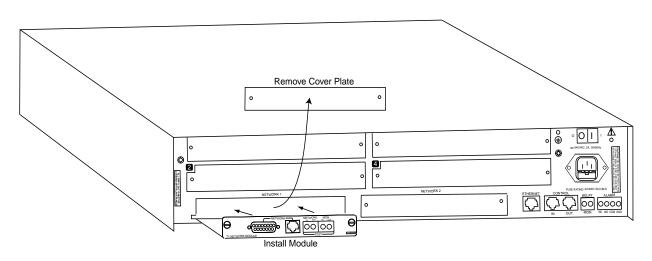
Figure 1. Installing the T1 Network Interface Module
